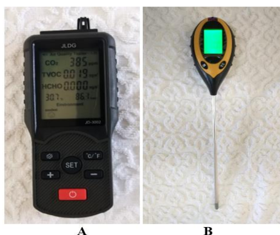
Figure 2. Digital measuring devices: (A) Carbon dioxide and temperature (B) Soil pH
